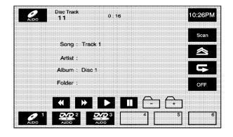
With the six-disc CD/DVD changer, you can play up to six audio CDs, MP3s, DTS discs, audio DVDs, or video DVD discs continuously.
